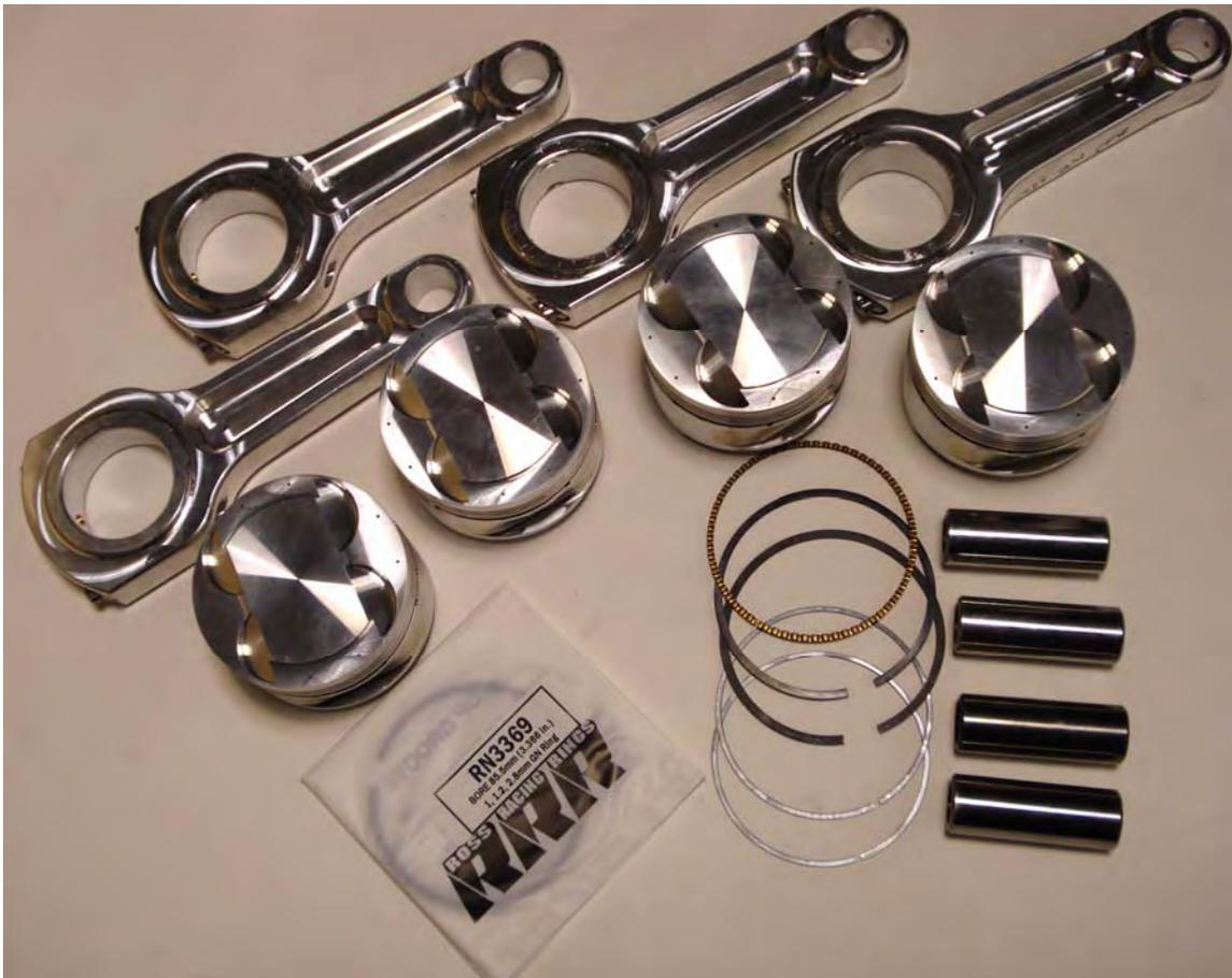
Magnus rods have an advanced profile and are built to withstand the torments of high hp and high RPM. Our Alloy rods feature L19 fasteners to allow for more clamp loading on the rod to survive at high RPM. They have been tested at over 350hp per cylinder. We recommend that any engine running over 800 HP should use our Aluminum Rods with our 23MM pin upgrade.
